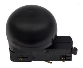
The controller performs two functions at one time: It creates a wireless CASAMBI network node and a wired DALI infrastructure supporting up to 8 addresses (Group or Short DALI Address). Included is a DALI power supply giving current for up to 50 luminaires.
